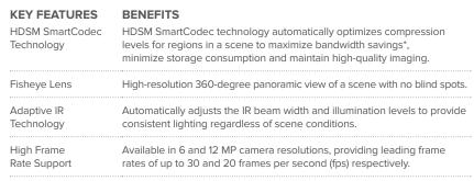
\*When activated, HDSM SmartCodec technology can reduce bandwidth by up to 50 percent compared to standard H.264 compression.
