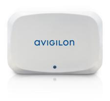
The APD™ is a sensor that combines self-learning analytics with impulse radar technology to detect the presence of a person with up to 99% accuracy, even if they have stopped moving or are hidden. This sensor is designed for indoor locations such as ATM rooms and other closed indoor vestibules within banks, pharmacies, retail stores and health care facilities.
